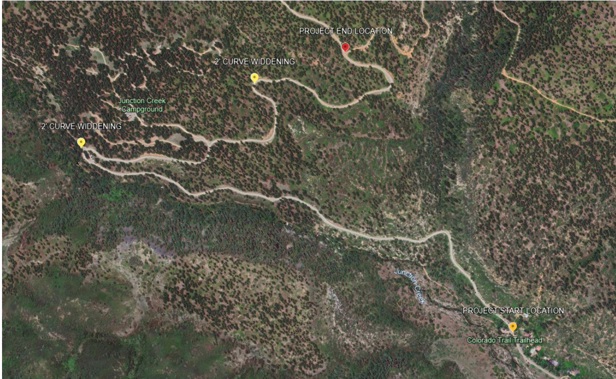
Project Overview – Road Reconditioning and Tripple penetration chip and seal from Colorado Trail head 1 to Log Chutes Trailhead 2.15 miles.
