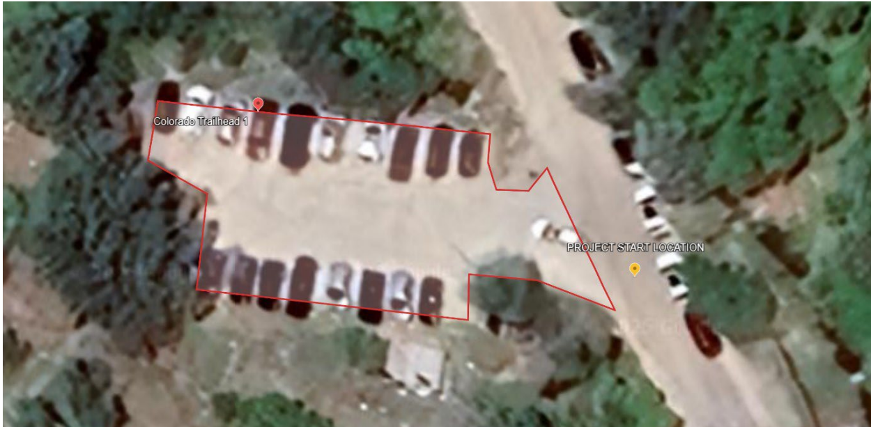
Colorado Trailhead 1 – Maintain surface, compact and surface with 3 layers of \frac{3}{4} " chip and seal. (5,750 square feet)
