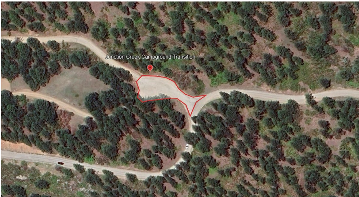
Junction Creek Campground Transition – Maintain surface, compact and surface with 3 layers of \frac{3}{4} " chip and seal. (10,850 square feet)
