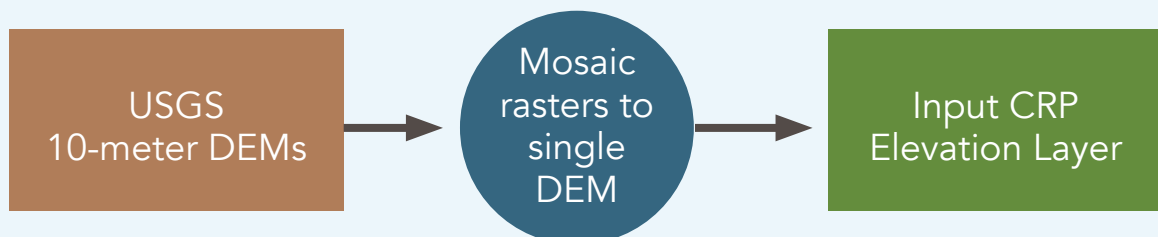
Figure 4: DEM Processing for Input Elevation Layer
